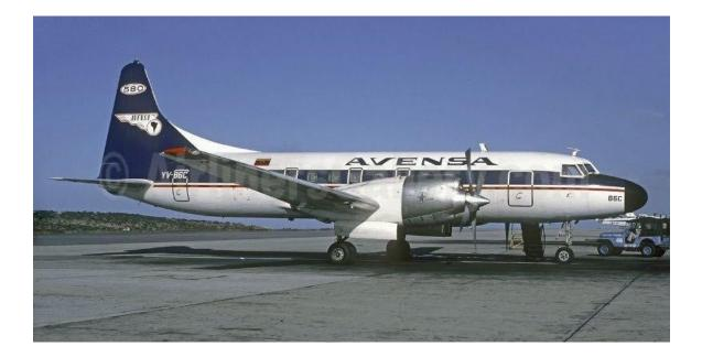
These TURBO-PROP powered Convairs were what the PDK refueling crew THOUGHT they were servicing: airplanes <u>that had been converted</u> and required jet fuel.
