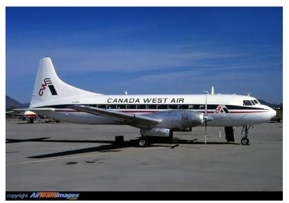
Others were converted to Allison turboprop engines, similar to those powering the Lockheed Electra and Navy P-3.
